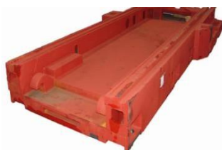
Cast iron frame for high stability in machining process.
