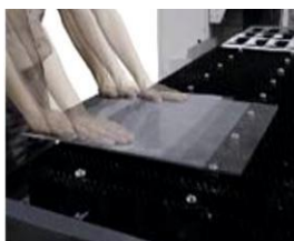
Work piece lifters help position material without damaging the bottom surface
